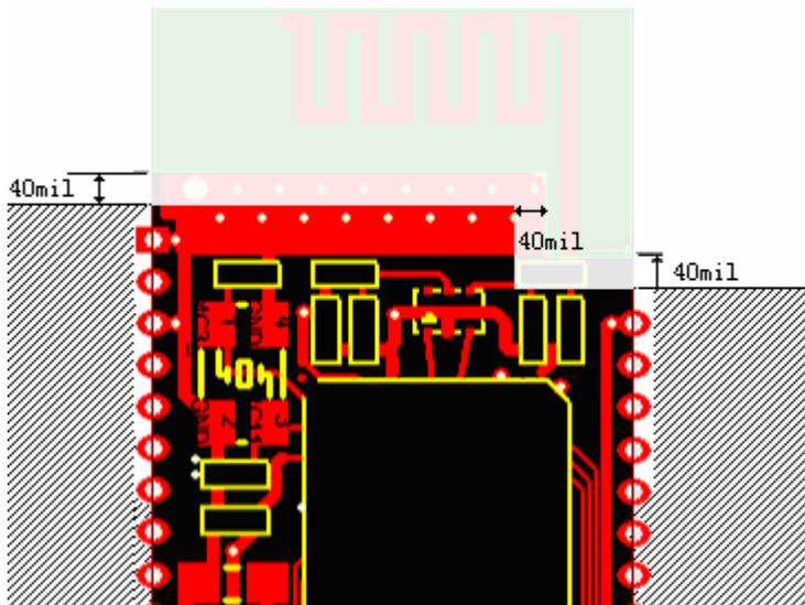
As you see above, trying to remove metal under antenna is good for RF radiate.
